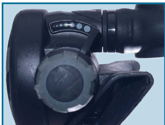
Rapid-adjustment knob and, above it, the venturi-control lever.
