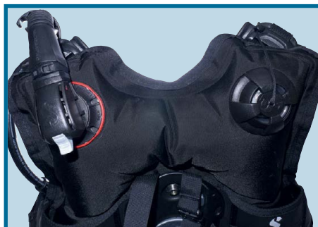
Rapid exhaust on the left can be activated by pulling down on the hose or depressing the switch on the elbow fitting.
