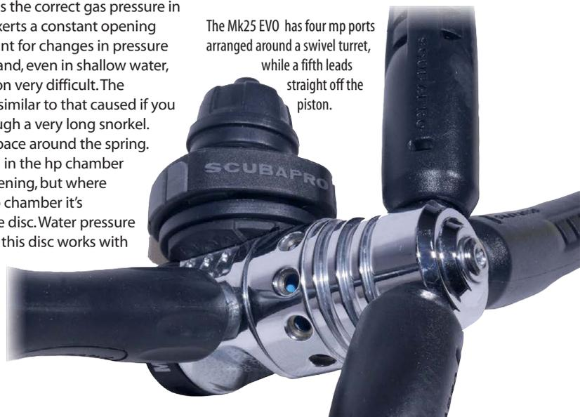
tank pressures. In the Mk25 EVO's balanced design air surrounds the piston, but doesn't act directly on it, so changes in tank pressure have almost no effect on breathing effort even when your cylinder is near empty.
