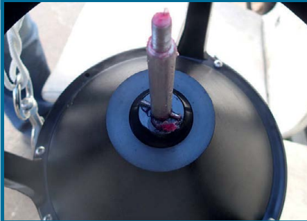
Propeller with twist-off cap, making it easy to remove under water even with gloves, and shroud.
