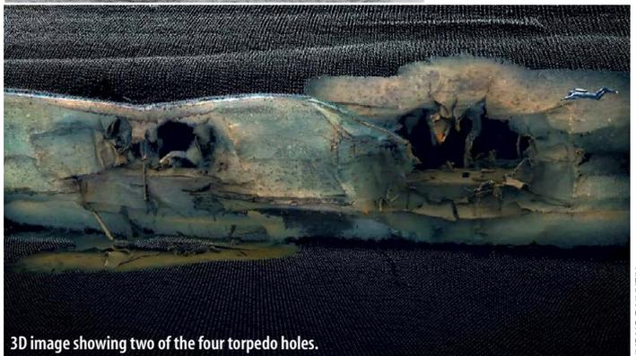
3D image showing two of the four torpedo holes.
